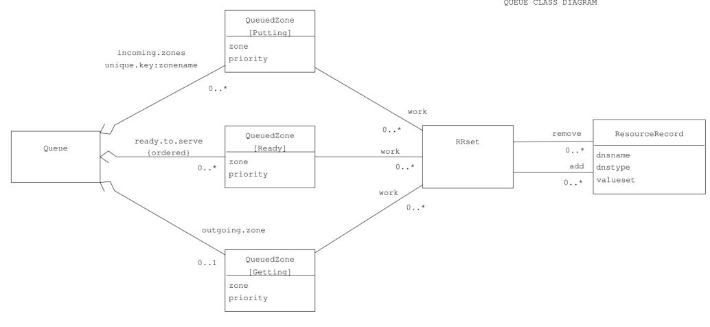
Much of the DNS workflow hinges on the Queue's operation. Internally, the Queue holds QueuedZones which list zone updates. The [states] refer to the state diagram for the QueuedZone, and instances move accordingly in this diagram when the proper (un)lock operation works on the Queue.
